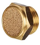
The silencer cap with sintered pad condenses the vapours present, making them fall back inside the tank. - Body in brass OT 58.
