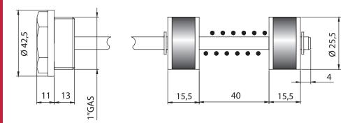
The probe cap with several elements and magnetic arc closing is the equivalent in characteristics to a magnetic column, but more economical.
