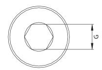
The hexagon socket head plug is useful when good tightening torque is required while avoiding protrusions.
