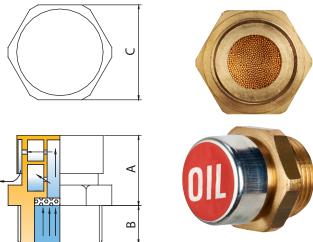
This range of oil breather caps has the same constructional characteristics as the TCSL, with the addition of a sintered bronze washer in the bottom part of the vent chamber, making it suitable for a "heavier duty" and therefore suitable for reduction units, overdrives, building machinery, road machinery, etc.
