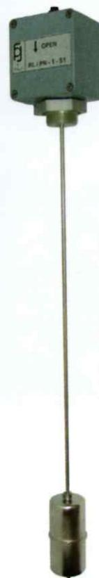
tural features give the IEG-CRXI a number of advantages: constant and continuous linear level indication with high precision of repeatability; linear level indication, regardless of the shape of the tank and the distance between the gauge and the tank walls; remote measurement indication and the possibility of piloting additional controls; accuracy of 12 mm; can be used in many dif-
